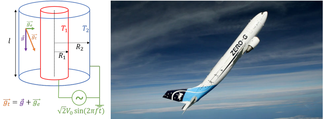
Figure 1: Schematic representation of the flow configuration (left) and photo of the A310 ZeroG airplane (right, by courtesy of Novespace).
