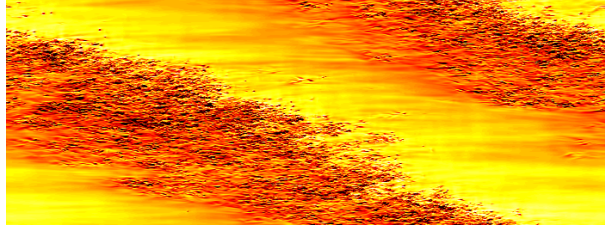
Figure 1: Streamwise flow field on the stable channel side in a plane parallel and close to the wall at Re = 20\,000 and Ro = 0.45 .
